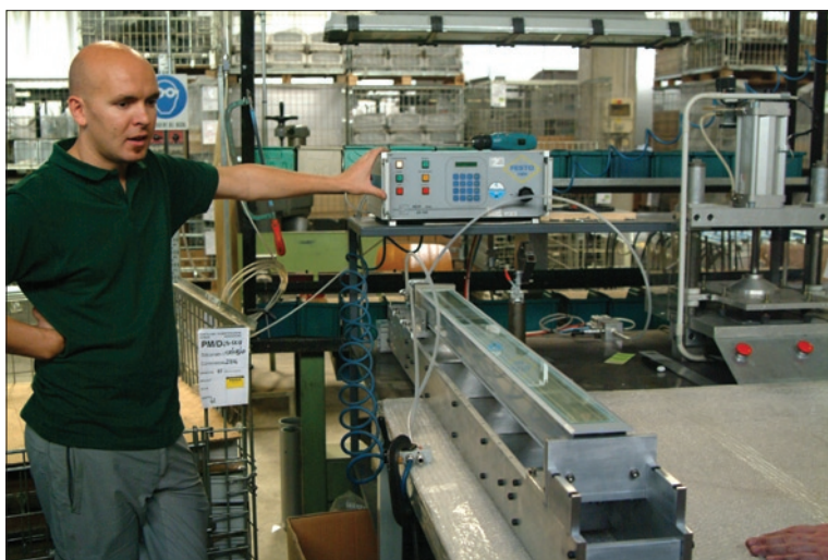
Obr. 6. Tlakové testy IP svítidel D49 NASTER – ing. Castaldi
