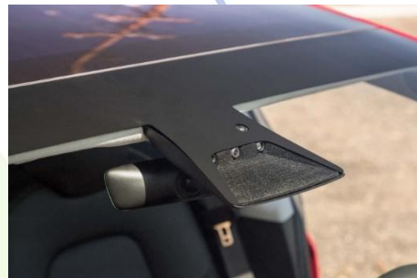
Main Forward Camera Max distance 150m
