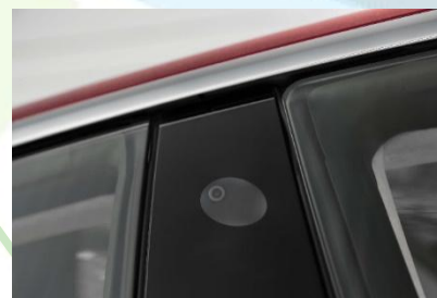
Forward Looking Side Cameras Max distance 80m
