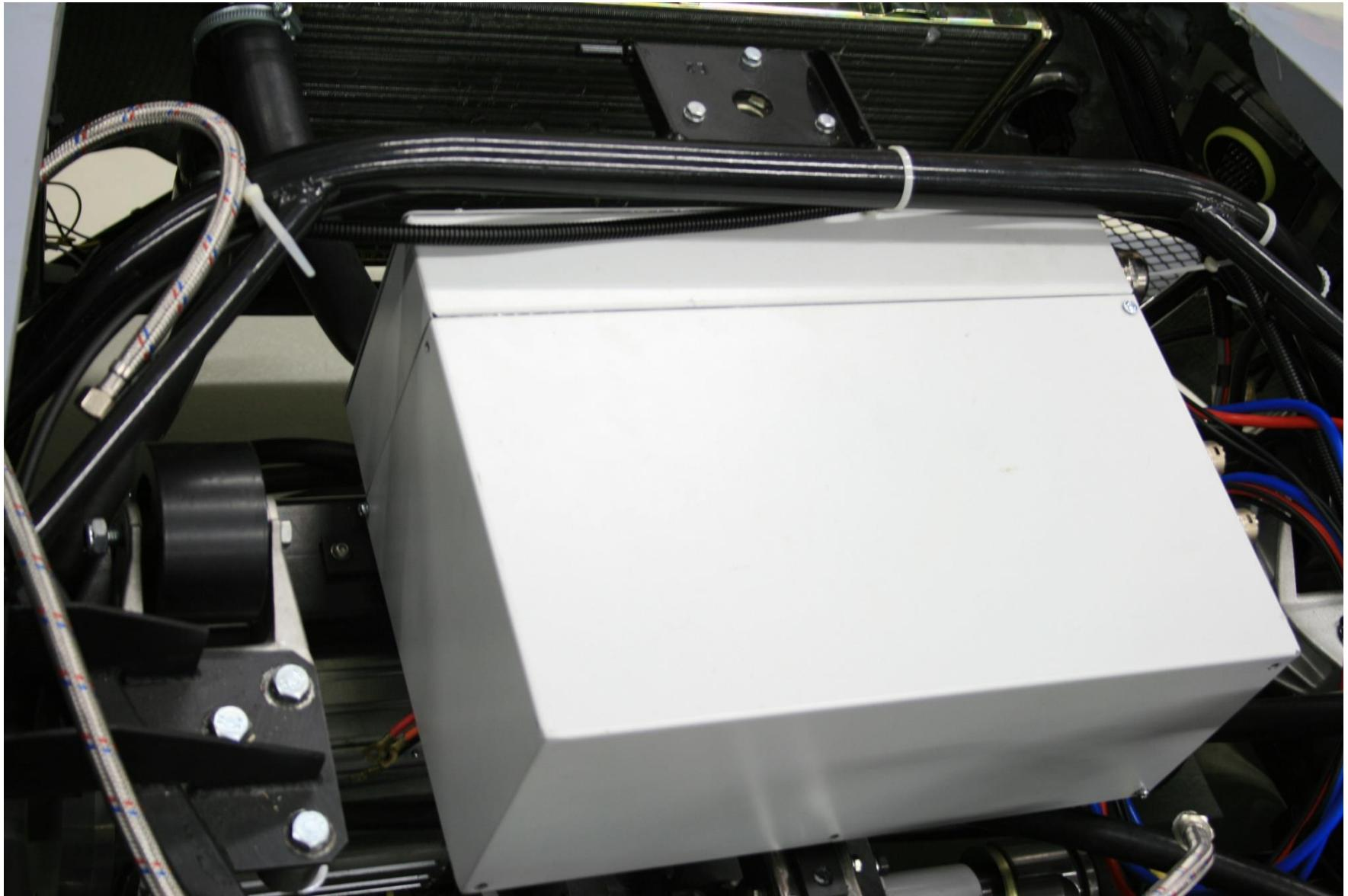
Fig.11. Twin DC/AC control unit VSB-TUO, chassis K1 (2011) and K0 (since 2012).
