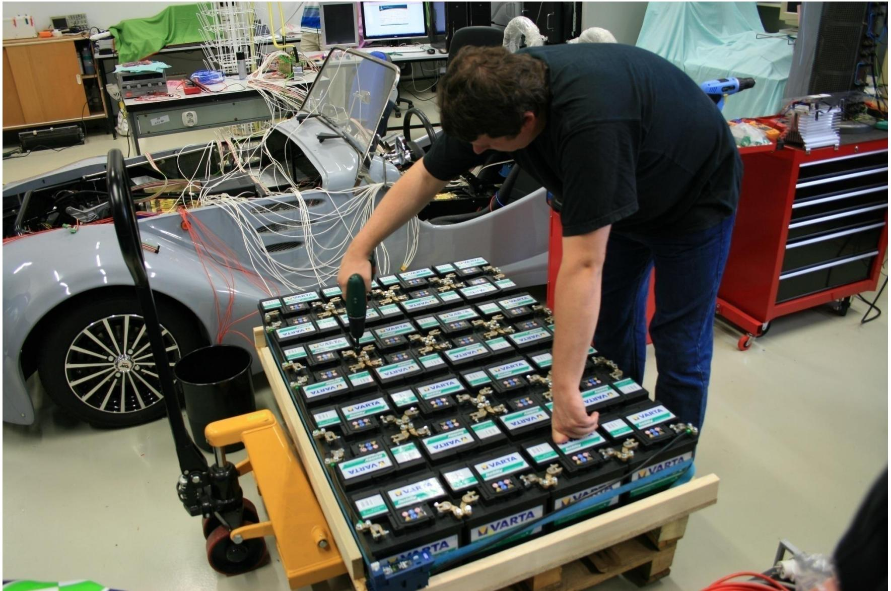
Fig.18. Experimental tractions battery 350V/40Ah (2010-2012).
