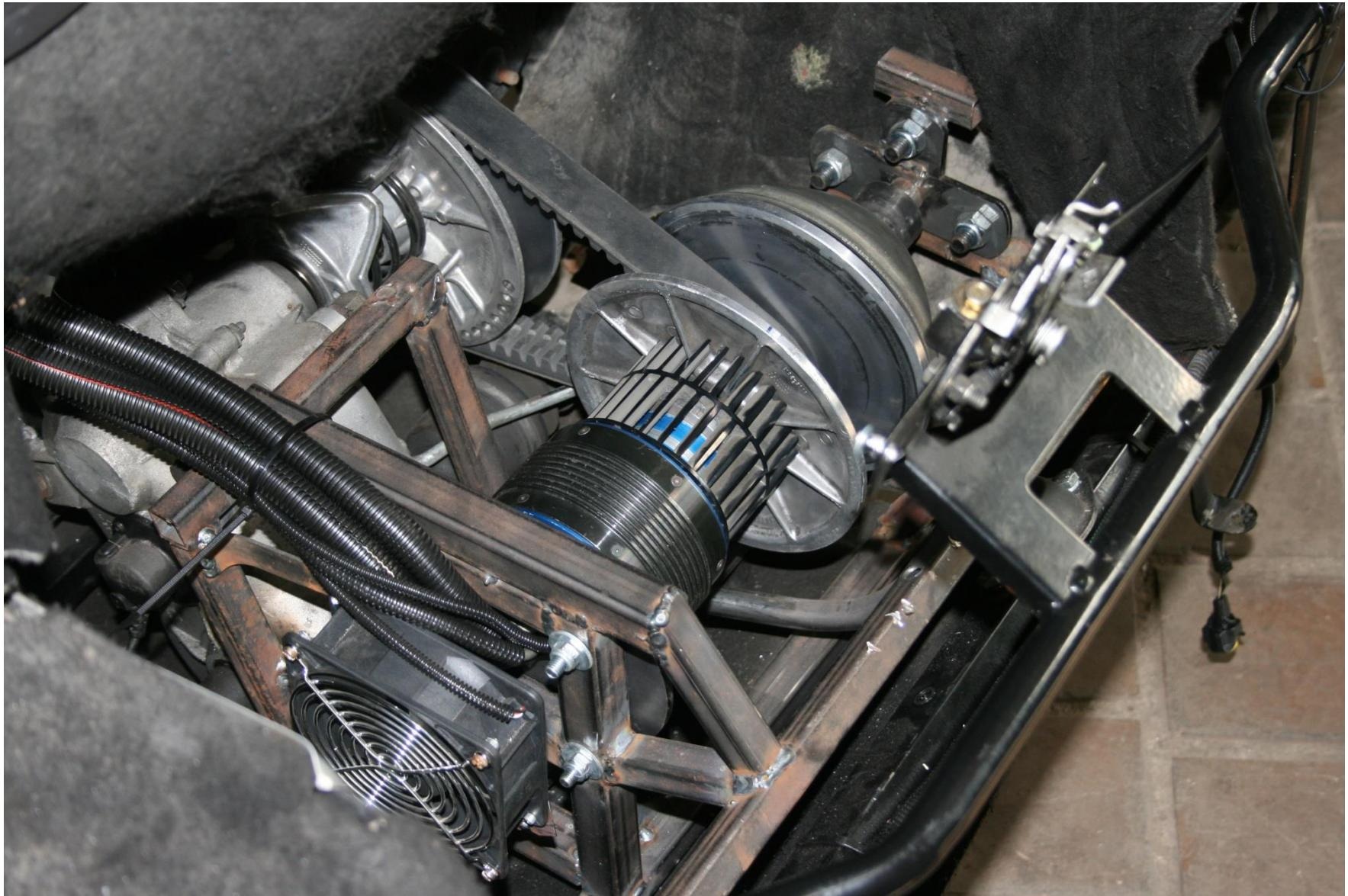
Fig.9. BLDC drive unit in chasssi AIXAM (2011).
