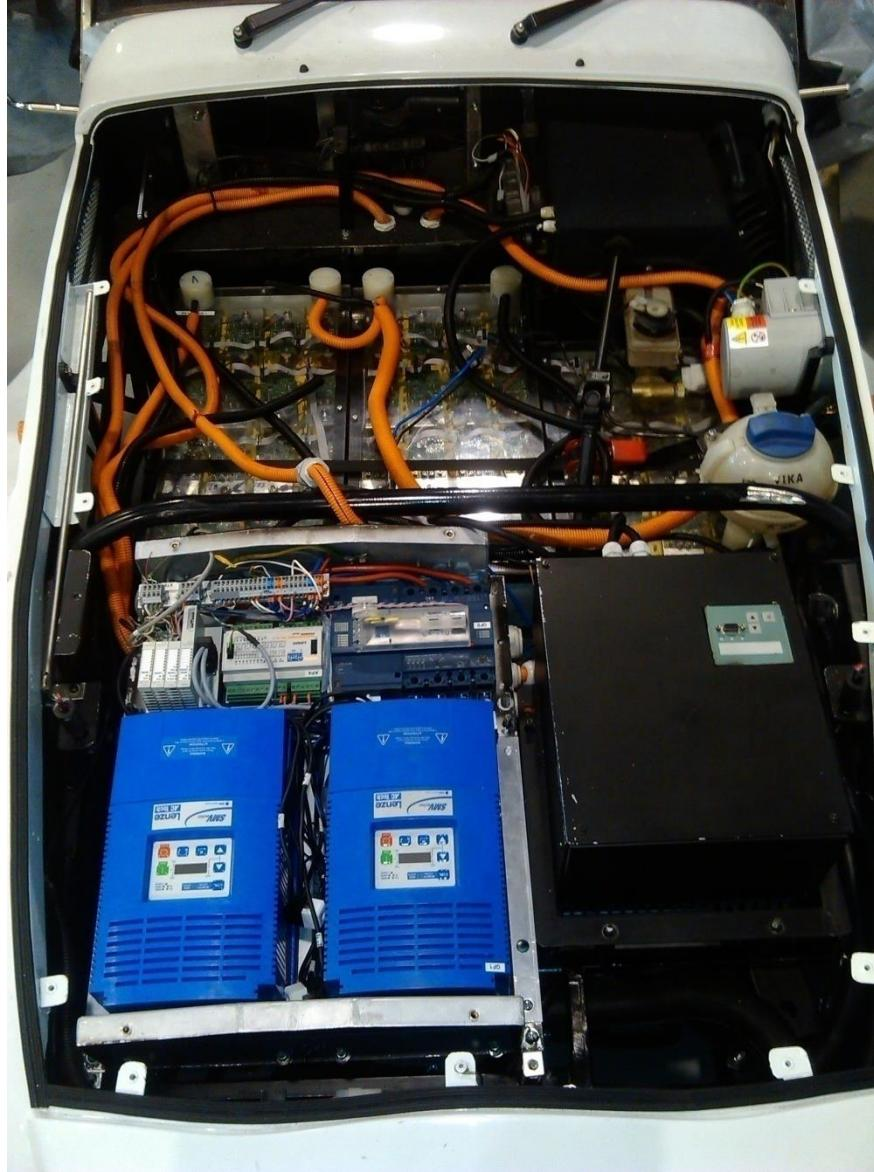
Fig.20. Charging implementation in the chassis K2 (black box right, 2011).
