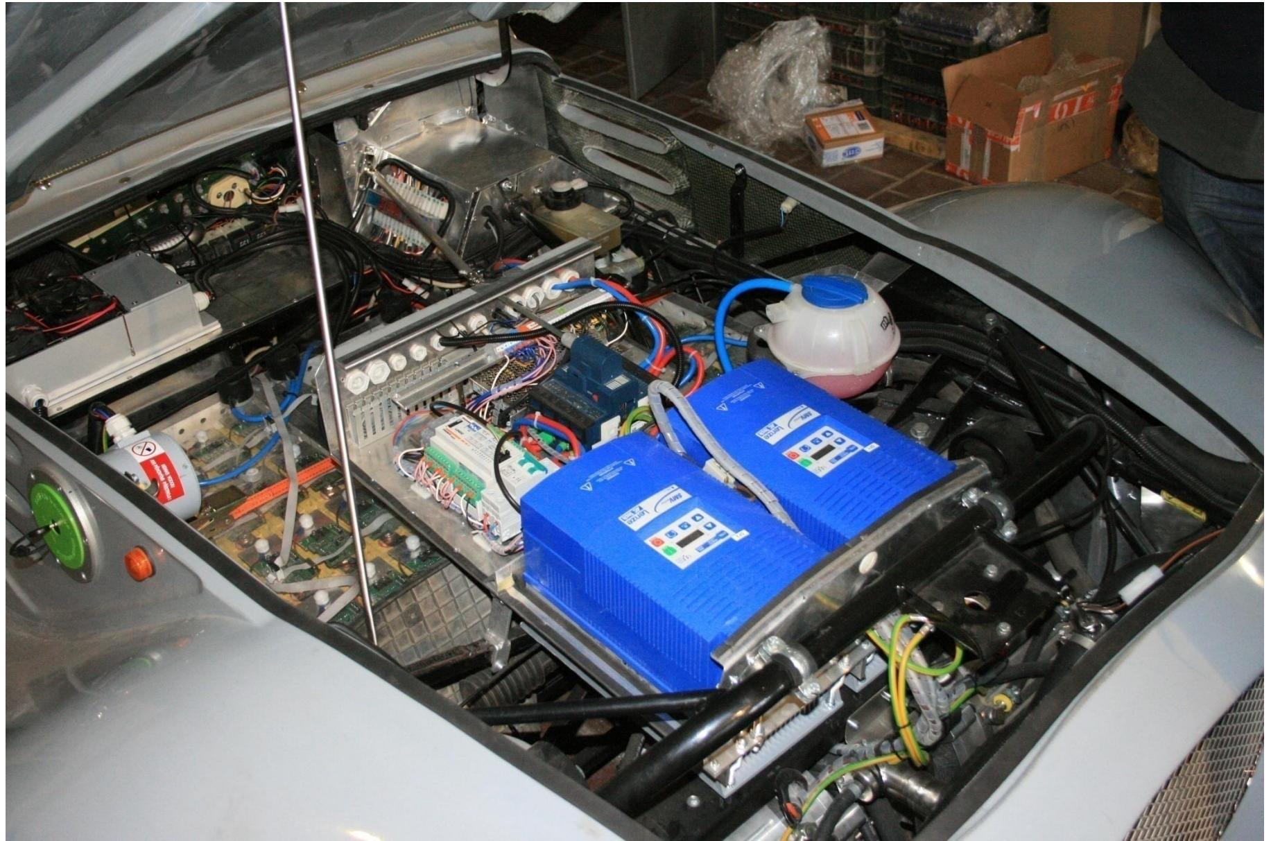
Fig.12. Implementation DC/AC Lenze control unit for K1 and K2 prototypes (2010/2012).
